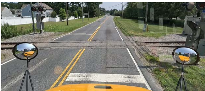
3. Come to a full and complete stop. Stop no closer than 15 feet from the crossing.
